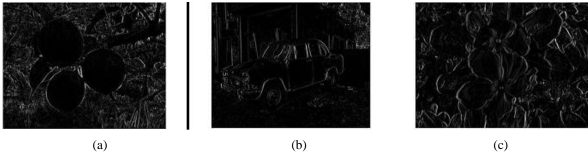
Figure 10: Gradient Images by Applying 7x7 LOG Filter (a) Gradient Image of Fruits by Applying 7x7 LOG Filter (b) Gradient Image of Car by Applying 7x7 LOG Filter (c) Gradient Image of Flowers by Applying 7x7 LOG Filter
